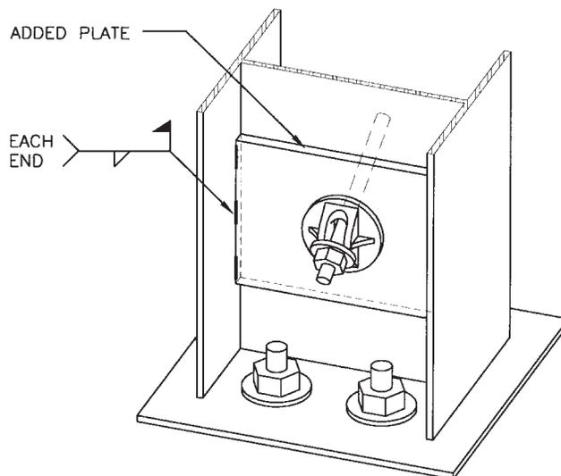
FIGURE 3.17 Added plate is used for web reinforcement.
